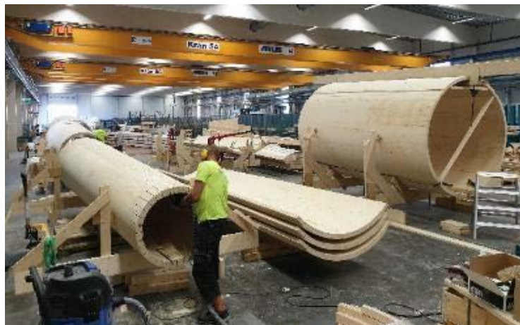
Figure 26 Manufacturing of the 30m Modvion prototype tower
